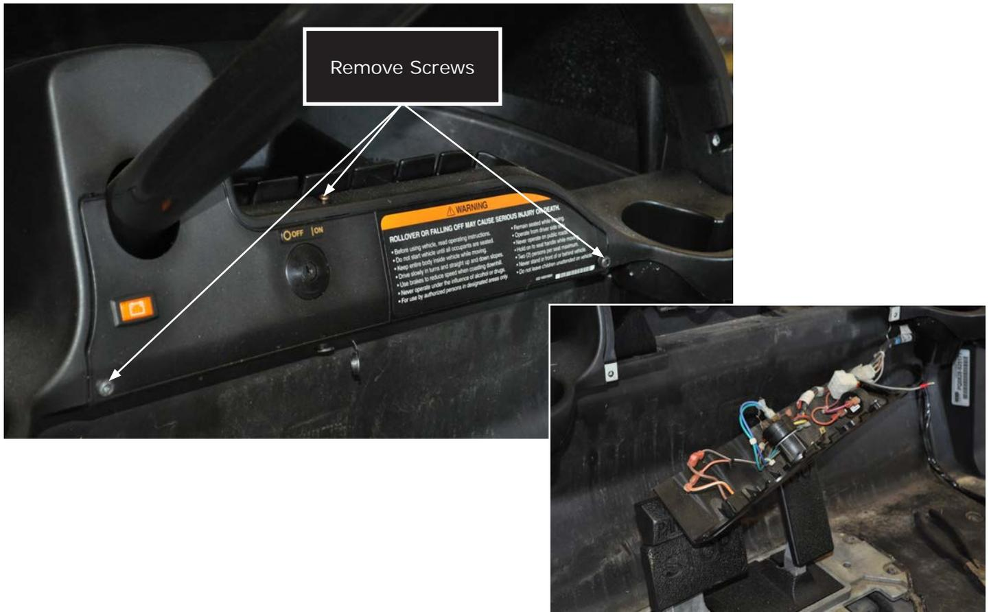
14. Following the path of the main harness, feed the 12-pin connector portion of new harness along the floor channel on passenger side of vehicle and up under the dash. Connect the red male bullet connector (gray wire) on the new harness to the red female bullet connector (gray wire) on the existing harness.
