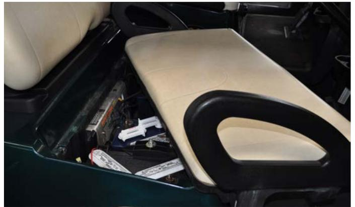
3. Place RUN/TOW switch in the TOW position
