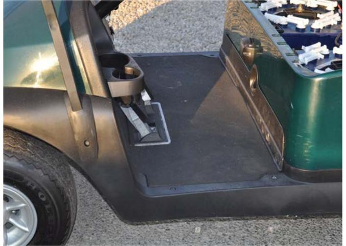
6. Remove the brake adjustment access panel.
