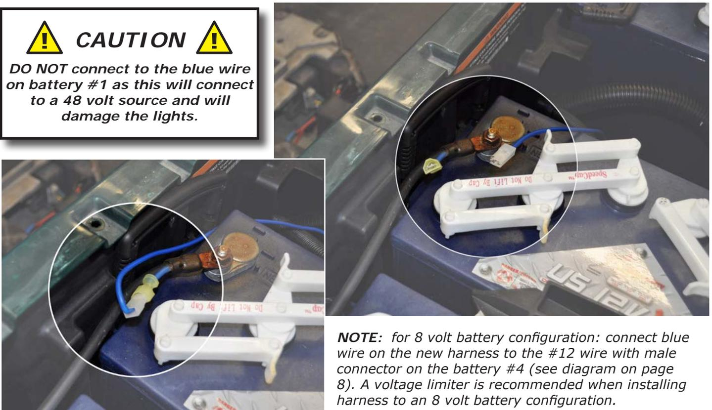
**NOTE:** for 8 volt battery configuration: connect blue wire on the new harness to the #12 wire with male connector on the battery #4 (see diagram on page 8). A voltage limiter is recommended when installing harness to an 8 volt battery configuration.
