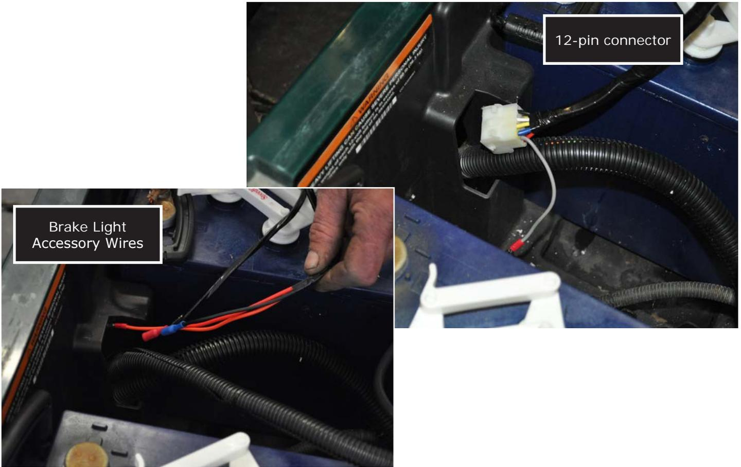
12. Follow the path of the existing main harness and pull Brake Light Accessory Wires through the center floor channel that leads to the brake compartment.
