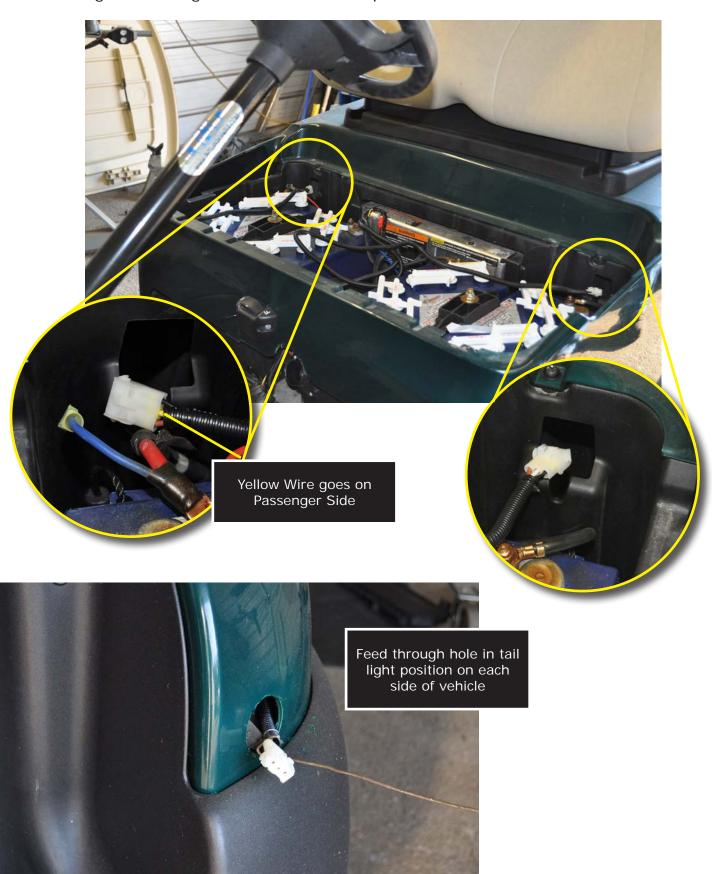
16. Behind battery #3 (see illustration) is a black #12 wire with a yellow female bullet connector. Connect the yellow male bullet connector on the new light harness with this yellow female bullet connector.
