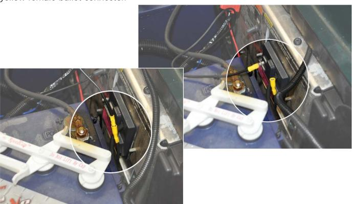
17. Connect blue wire on the new harness to the #12 wire with male connector on the battery #3 (see diagram).
