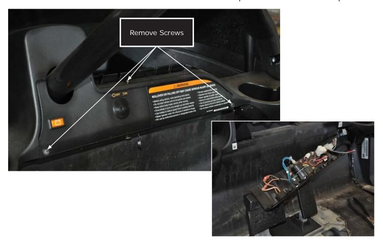
14. Following the path of the main harness, feed the 12-pin connector portion of new harness along the floor channel on passenger side of vehicle and up under the dash. Connect the red male bullet connector (gray wire) on the new harness to the red female
