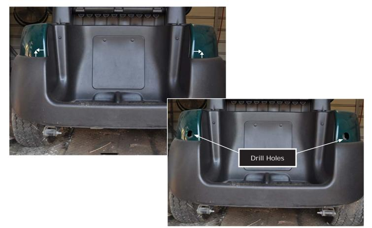
11. Thread the 12-pin connector and Brake Light Accessory Wires from inside the battery compartment through the hole where the existing main harness feeds.
