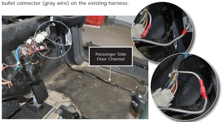
15. Using a wire snake or fish tape (not supplied), route the tail light wires through the holes in the upper corners of the battery compartment on both the passenger's and driver's sides. The passenger's side has the yellow wire in the 3-plug connector. Feed the snake through the tail light holes drilled in Step 10.
