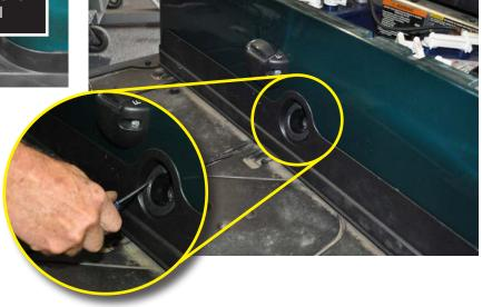
9. Remove and retain the three screws that secure the lower body trim to the body and lift off the lower body trim.
