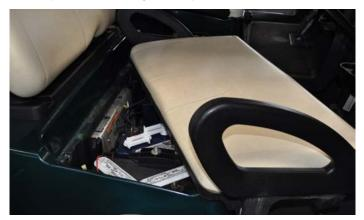
3. Place RUN/TOW switch in the TOW position
