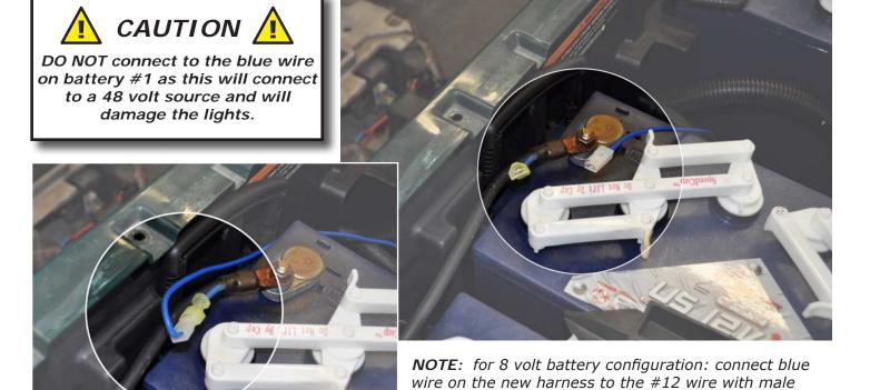
connector on the battery #4 (see diagram on page 8). A voltage limiter is recommended when installing
