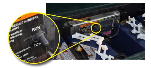
4. Disconnect the wire from the negative terminal on battery #4 on the driver's side. (See Battery Diagram on the last page of these instructions)
