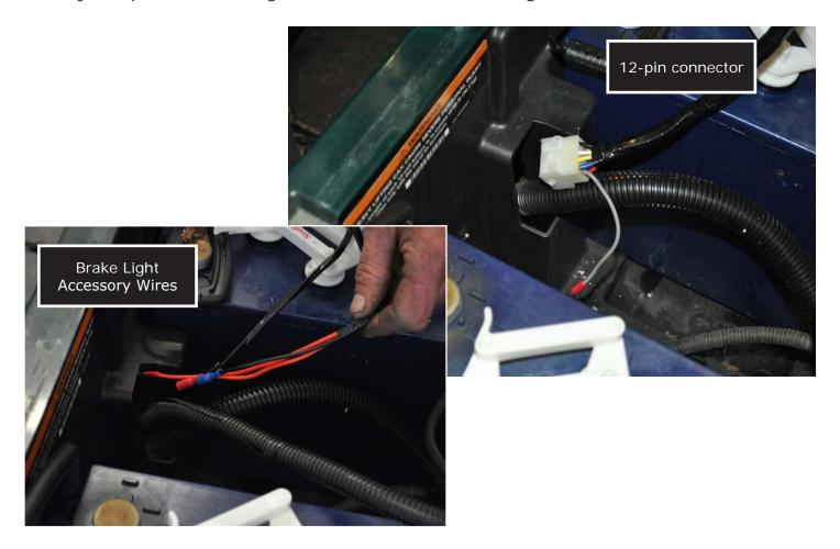
12. Follow the path of the existing main harness and pull Brake Light Accessory Wires through the center floor channel that leads to the brake compartment.
