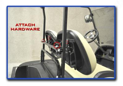
Attach seat back to seat back brackets using hardware from step 3. Attach seat back brackets to seat back bar using 45mm bolts from hardware pack 2.
