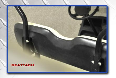
Reattach seatback using hardware from step 2.
