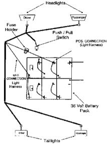
E-Z-Go Basic 36-Volt Wiring Diagram
