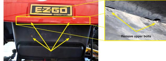
1. Remove the four factory bolts from the bumper guard housing. *Retain hardware*.
