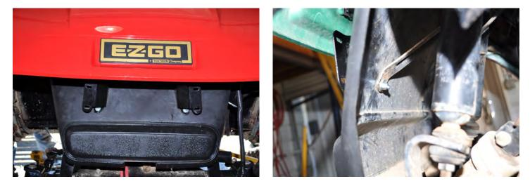
3. Install Light Bar to Mounting Brackets.
