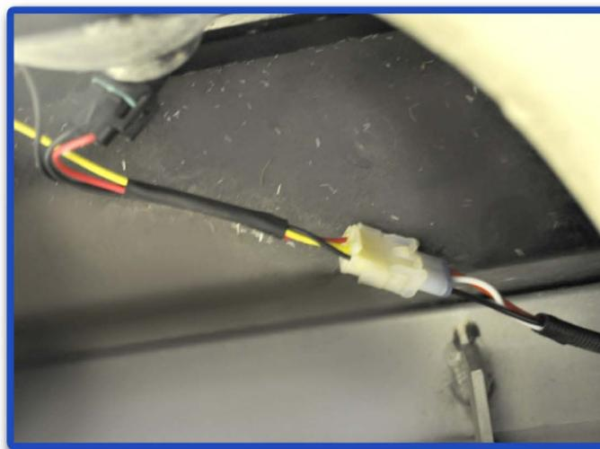
Plug headlights and tail lights into harness as shown.
