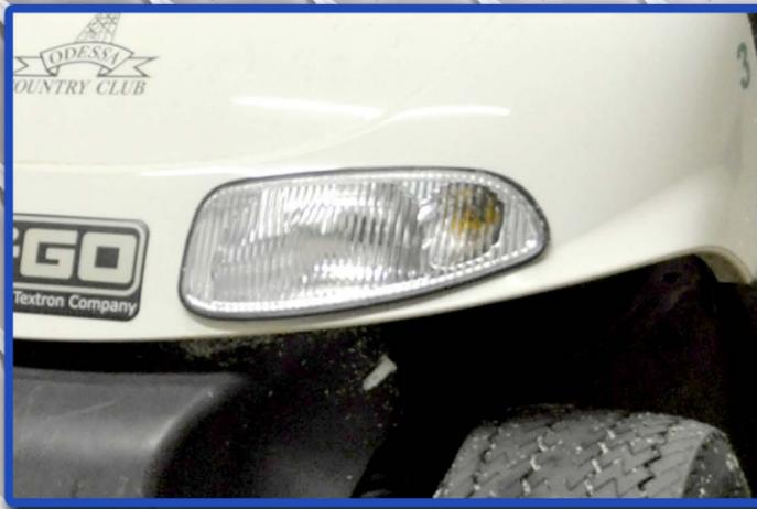
Insert headlight and attach to cart using clips located behind the headlight.
