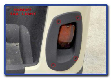
Cut out template and place it against cart using the body lines for alignment.
