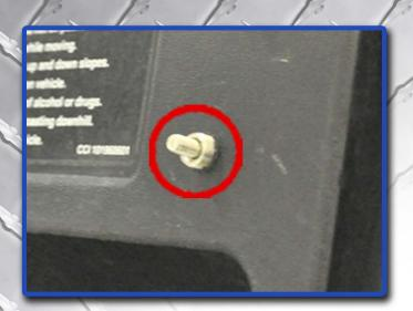
Feed threaded end of switch through the dash where the hole was drilled. Attach the nut to secure the harness.
