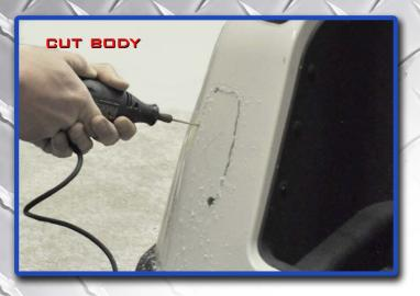
Using the template you drew on the cart, cut out the light area of the body starting at the pilot hole from step 2.
