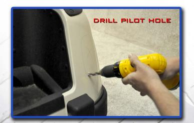
Draw the inside of the template out with a writing utensil. Next drill a pilot hole so you will have a starting point to begin cutting.
