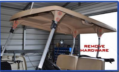
Remove lower strut bolts and remove rear struts. If installing a seat on a Yamaha G-22, retain rear struts for later use.
