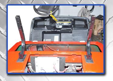
Insert main brackets into holes where OEM front seat supports were removed. Be sure the tabs are pointed to the cart's CENTER, as shown. Secure the main brackets with hardware retained in step 6.
