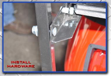
Attach seat frame to rear portion of armrest using hardware from pack 2. Be sure to place hardware as shown.
