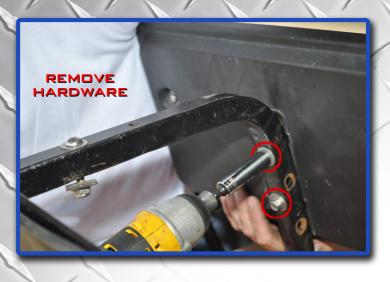
Remove OEM front seat backs. Retain hardware.
