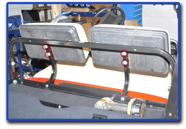
Reinstal front seat backs using hardware retained in step 3.
