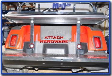
Attach footrest to bagwell bracket using remaining hardware from pack 1.
