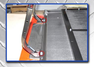
Place seat frame on cart. Attach seat frame to main brackets using hardware from pack 1.
