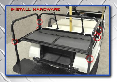
Attach seat back support and armrests using hardware from pack 3.
