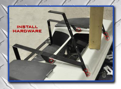
Install main seat frame brackets and front seat lean back brackets to front with retained hardware. Using 8mm hardware from pack 1, mount middle bracket to cart.
