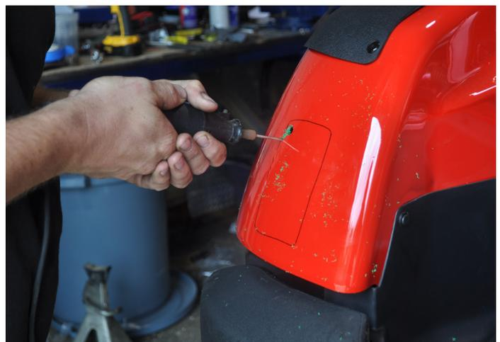
14. Route wiring harness behind rear fender wells. Attach rear lights and mount to bodywork using supplied screws.
