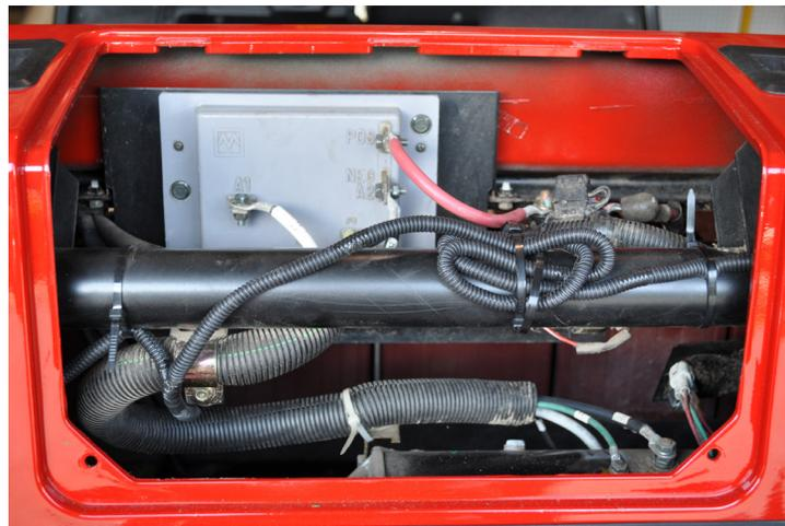
**IMPORTANT:** How you connect the wiring harness to your cart's battery pack will depend entirely on your cart's battery pack configuration. This light kit is intended for 12 Volt applications. Take care not to supply too much voltage to the unit as this will cause a failure that is not covered by manufacturer's warranty.
