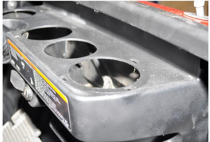
3. Locate a place on the dashboard to mount the switch. We recommend using the location shown as it does not interfere with the cup holder when reinstalled and also allows you to easily route the wiring harness.
