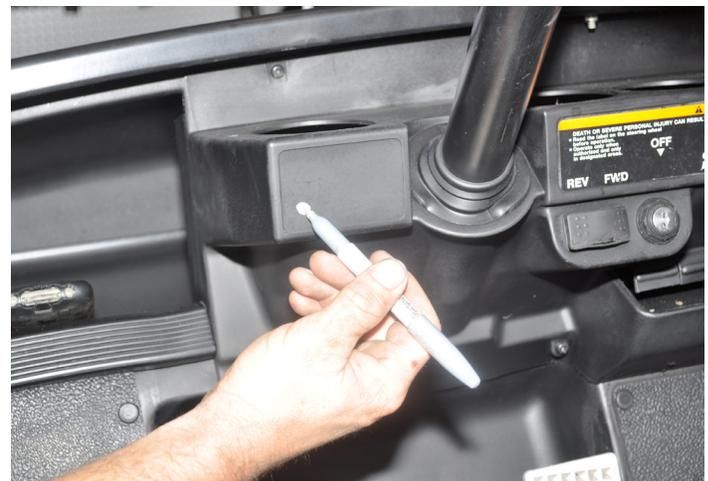
4. Select a drill bit size that is as close to the diameter of the exposed portion of this switch as possible and drill at location marked in **Step 3**.
