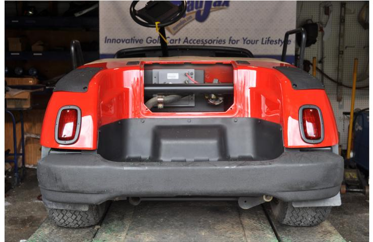
15. Use the supplied zip ties to fasten wiring harness to vehicle. MadJax recommends fastening the wiring harness to frame members in the front of the vehicle in order to prevent the harness from making contact, rubbing, or being pinched by moving parts, such as the suspension. Use two zip ties to tie the wiring harness to the frame at the back of the motor compartment as shown. Replace motor cover.
