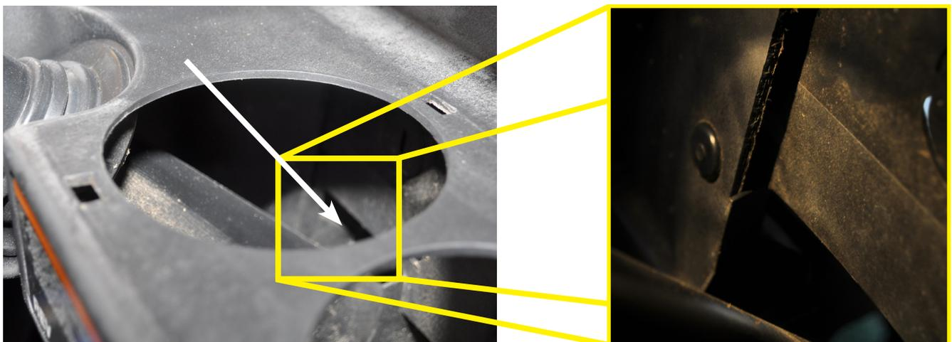
7. Cut out Headlight Template and tape to bodywork as shown. For best results, ensure the center most edge of the template is aligned with the bodywork's geometry. Mark cutout with a Sharpie or other permanent marker. Simply flip the template over to do the other side.
