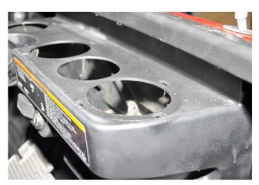
3. Locate a place on the dashboard to mount the switch. We recommend using the location shown as it does not interfere with the cup holder when reinstalled and also allows you to easily route the wiring harness.
