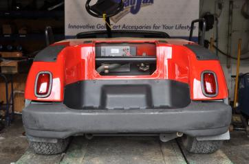
15. Use the supplied zip ties to fasten wiring harness to vehicle. MadJax recommends fastening the wiring harness to frame members in the front of the vehicle in order to prevent the harness from making contact, rubbing, or being pinched by moving parts, such as the suspension. Use two zip ties to tie the wiring harness to the frame at the back of the motor compartment as shown. Replace motor cover.
