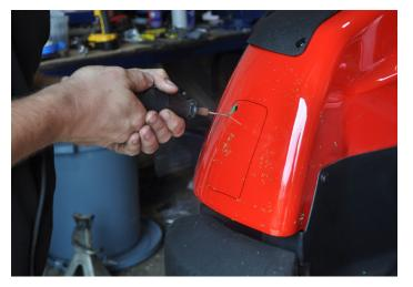
14. Route wiring harness behind rear fender wells. Attach rear lights and mount to bodywork using supplied screws.
