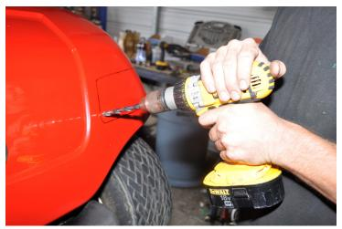
9. Drill a pilot hole and cut out bodywork.
