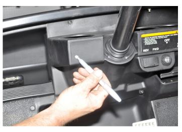
4. Select a drill bit size that is as close to the diameter of the exposed portion of this switch as possible and drill at location marked in **Step 3**.
