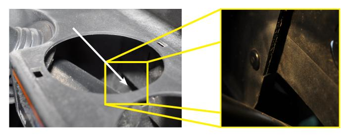
7. Cut out Headlight Template and tape to bodywork as shown. For best results, ensure the center most edge of the template is aligned with the bodywork's geometry. Mark cutout with a Sharpie or other permanent marker. Simply flip the template over to do the other side.
