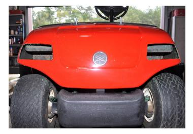
10. Place headlight assemblies into cutouts and attach to wiring harness. Fasten headlight assemblies to cowling using the supplied screws.
