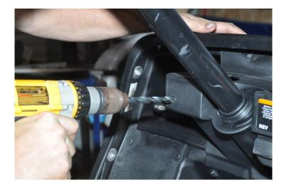
5. Mount the switch through the hole and attach to dashboard using the switch's trim ring.
