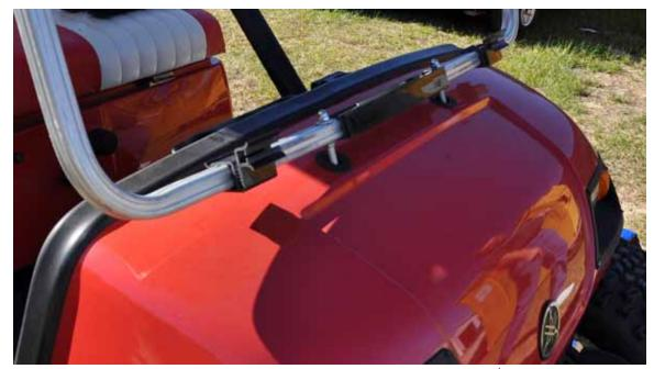
2. Attach Windshield Strut Clamps to Windshield Strut as shown. Center clamps between bends in Windshield Strut and hardware that secures Windshield Strut to vehicle.
