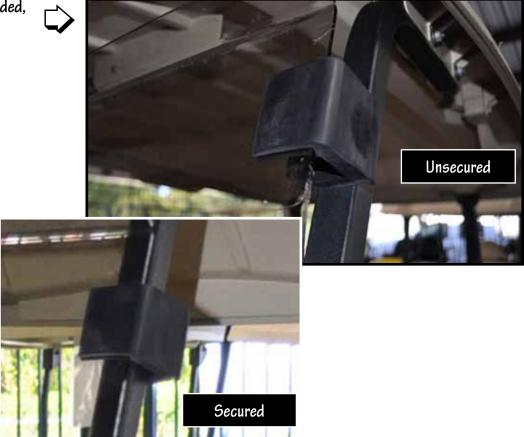
7. Squeaking may occur, caused by friction between windshield and strut bracket. Application of a spray lubricant (such as WD-40) down channels of Windshield Strut Brackets, should minimize this.
