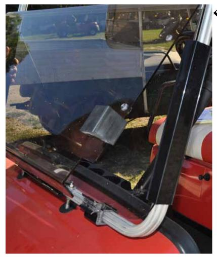
] 5. Attach lower ends of Long Windshield Strut Brackets to Windshield Strut and slide bottom of Windshield into channels of Short Windshield Strut Bracket and Windshield Strut Clamps. 6. To secure winshield when unfolded, use clamps on upper portion of windshield.
