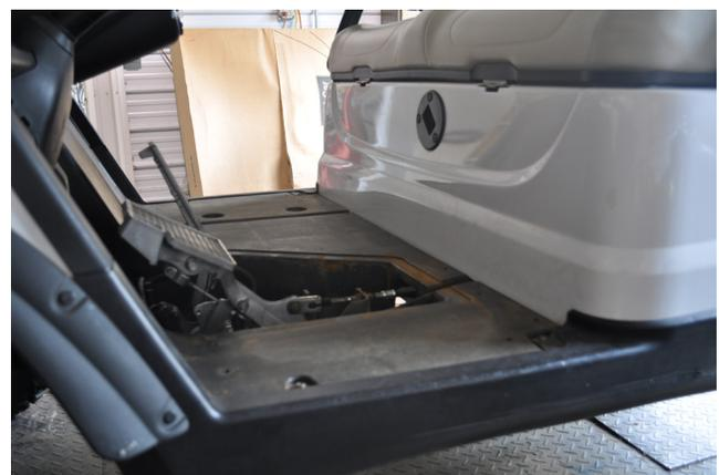
4. Route wiring harness through pedal assembly area to areas for headlights and tail lights. Route wiring harness through dash to a location to mount headlight pull switch.
