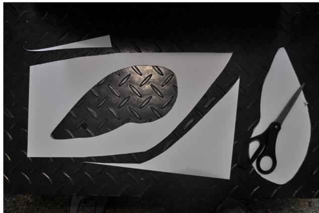
5. Align template to front cowling contour using the lower edge of the cowling as shown. Trace the inside of the cutout to mark the headlight position using a permanent marker (e.g., Sharpie®). Once you have completed the right side, flip the template over and mark the left side.
