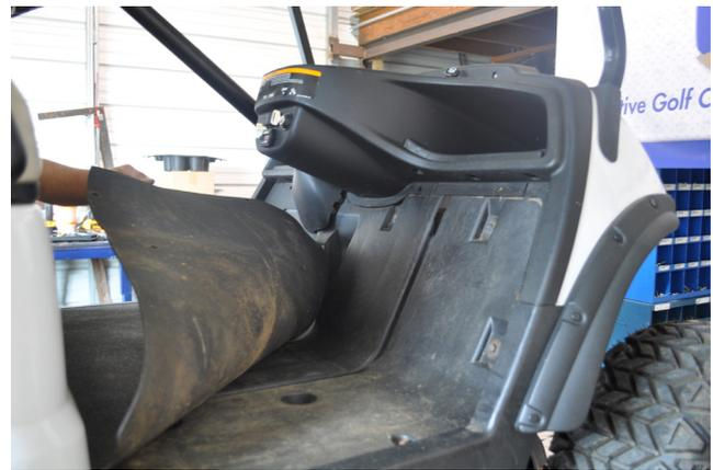
3. Lift plate from floor to expose pedal assembly.
