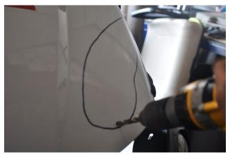
7. To cut the cowling, MadJax recommends the use of a rotary tool (such as a Dremel® or RotoZip®) and a bit specifically made for cutting plastic.
