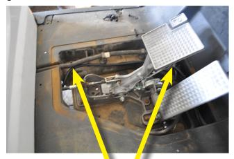
Zip Tie Locations (location at right of photo is *behind* brake pedal)
