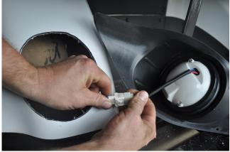
12. To fasten wiring harness to vehicle use the supplied zip ties. MadJax recommends fastening the wiring harness to frame members in the front of the vehicle in order to prevent the harness from making contact, rubbing, or being pinched by moving parts, such as the suspension. Use two zip ties in the pedal assembly area, as shown, to tie the wiring harness to the main wiring harness. Tie the wiring harness to the main harness at the back of the battery compartment as shown.
