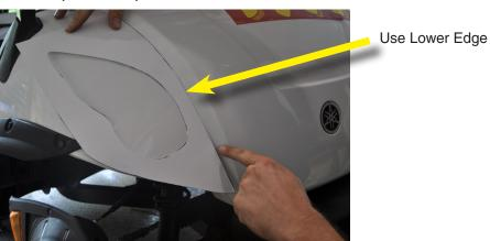
6. Drill pilot holes on the INSIDE of the marks as shown.
