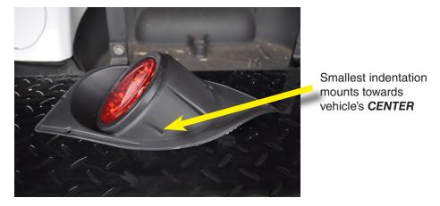
11. Route wiring harness behind rear fender wells. Attach rear lights and mount to cowling using supplied barbed plastic fasteners.
