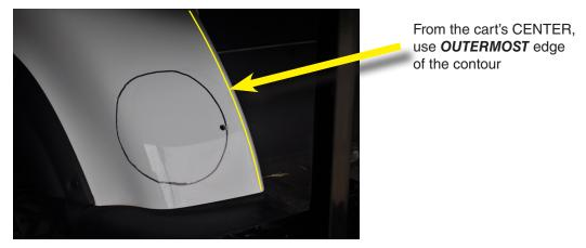
10. Drill a pilot hole and cut out cowling.
