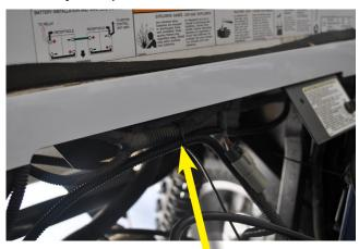
Zip tie to main harness at rear of battery compartment.
