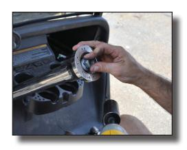
Remove horn switch assembly from MadJax steering wheel and press onto steering hub adapter, aligning the grooves with the holes in the adapter.
