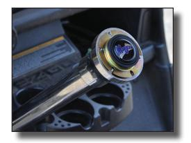
Press steering wheel onto horn switch assembly. Check hole alignment.
