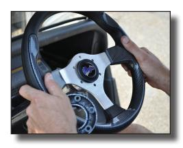
Attach trim ring and steering wheel to steering hub adapter using six included hex socket bolts.
