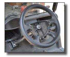
Loosen and remove nut from steering column spindle. Retain Nut.
