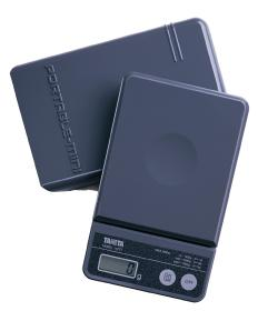
The 1475T is Tanita's highest capacity pocket scale. An electrostatic capacitance load cell makes this scale feather-touch sensitive up to 1,200 grams. Unique hard cover provides unsurpassed protection, while also serving as a gem tray when removed. Features a tare function with a clear 4-digit LCD display and 2 different modes of measurement: Gram and, Ounce. Measurement accuracy of I gram is achieved up to 500 grams, and 2 grams accuracy from 500 to 1,200 grams.
