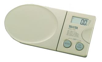
The 1479S uses an electrostatic capacitance load cell to provide highly accurate and repeatable measurements in a rugged package. Unique hard cover provides unsurpassed protection, while also serving as a gem tray when removed. Features a tare function with a clear 4-digit LCD display and 4 different modes of measurement: Gram, Ounce, Troy Ounce, and Penny Weight. A capacity of 300 grams, with a measurement accuracy of 0.1 gram.
