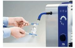
**Cleaning with fixed nozzle and foot pedal** Ideal for working with both hands or for larger workpieces.
