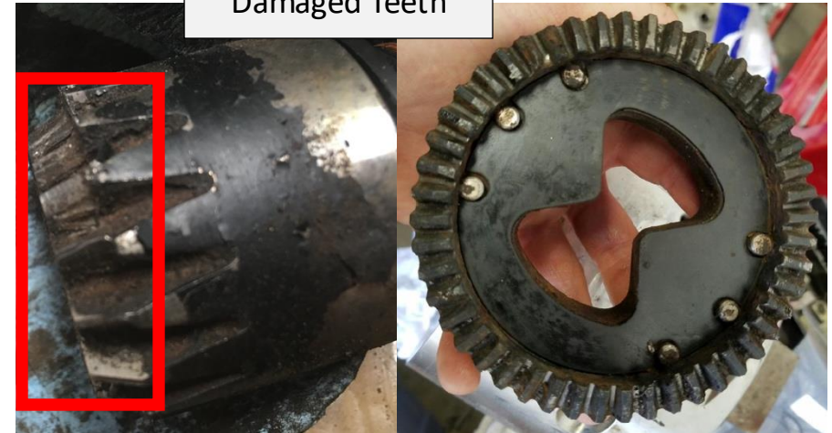
Classic Disc Choke Damage
