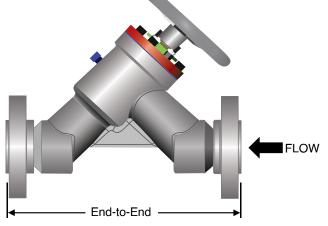
The MDIS Steam valve is designed for high pressure throttling of steam. The multiple orifice system is designed for long life in difficult applications. The standard valve has 1", 2", or 3" female NPT ends, with flanged or special ends readily available. Standard trim is Tungsten Carbide and designed for linear flow characteristics. Manual or electric actuation is standard.
