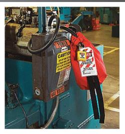
At Innovations Manufacturing only designated employees can lockout power sources and/or an alternative group lockout process is used.
