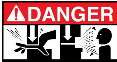
Moving slides and dies on POWER PRESSES can crush, dismember, snag, hit, and entrap, causing serious injury or death.
