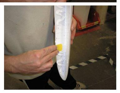
Apply the bumper to the bow using the pencil marks as a guide. It is important to avoid capturing air bubbles within the adhesive while applying the bumper to the boat, as trapped bubbles will decrease the contact area
