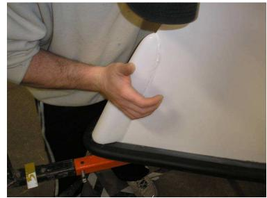
Scrape off the excess adhesive. Wet the rag liberally with acetone and use your finger to wipe the 4/5200 off the bumper. A few passes over the area will easily remove the excess 4/5200
