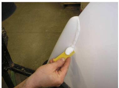
Cover, or otherwise protect, the area from exposure to water for the curing duration. In 75°F 24 hours are needed to cure; 60°F 36 hours, 45°F 50 hours. Secure the bumper to the bow with tape
