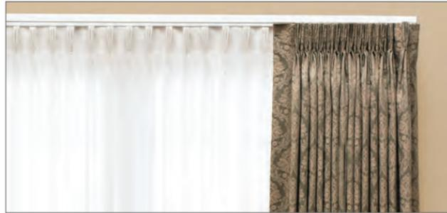
**Ripplefold** — named for the soft, consistent ripples created by the drapery as it hangs from the track. Fullness of the drapery is determined by the carrier spacing. Lutron ripplefold tracks are available in three fullness factors: 80%, 100%, and 120%.
