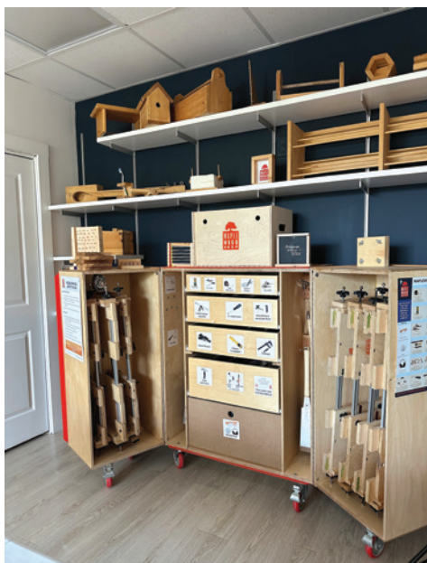
Schloff designed a portable woodworking system. His “shop class in a box” fits inside a lockable rolling tool chest. It includes tools, wood, lesson plans, safety protocols, emotional learning cues and a tray-like bench that sits atop a table.
