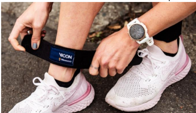
I Measure U is a lower-limb monitoring device. Courtesy, Dr. Peter Friesen
