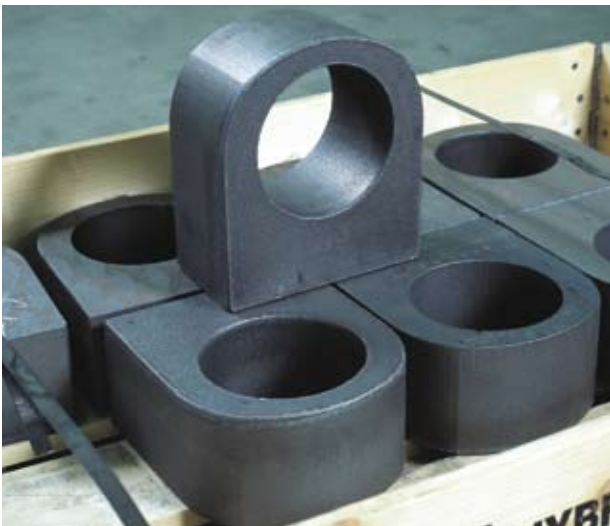
Flame cut blanks for a bearing house.
