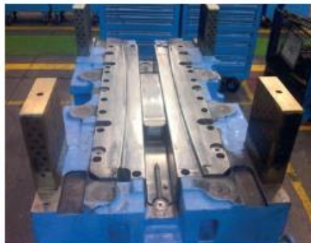
Pic.2: No segment (monoblock) on drawing edge.
