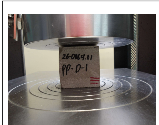
Photo No. 2 ASTM C170 – Compressive Strength Test Setup
