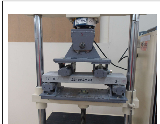
Photo No. 10 ASTM C880 – Specimen Loading Detail
