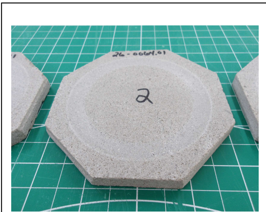
Photo No. 15 ASTM C1353 – Representative Post- Abrasion Specimen Condition
