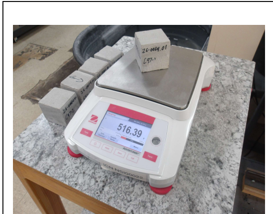
Photo No. 1 ASTM C97 – Test Apparatus (Dry Mass Determination Depicted)
