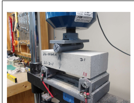
Photo No. 6 ASTM C99 – Specimen Loading Detail
