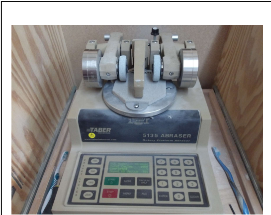
Photo No. 13 ASTM C1353 – Abrasion Apparatus
