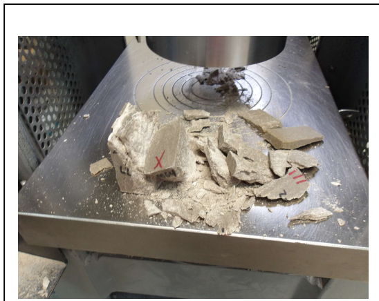
Photo No. 3 ASTM C170 – Representative Specimen Failure Mode (Parallel Loading - Wet Condition)
