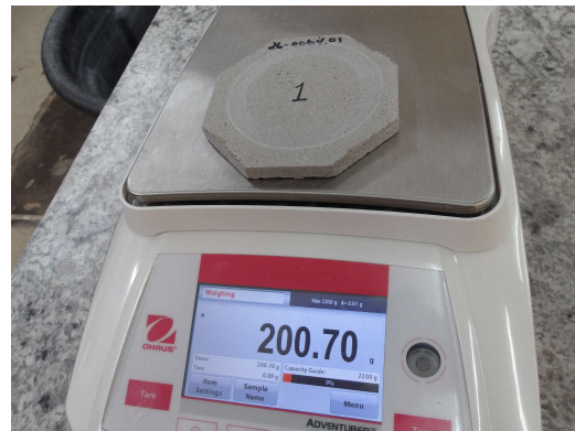
Photo No. 16 ASTM C1353 – Representative Post- Abrasion Mass Determination
