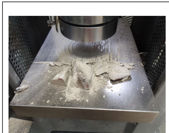
Photo No. 4 ASTM C170 – Representative Specimen Failure Mode (Perpendicular Loading - Dry Condition)
