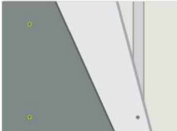
1. Interior Framed Wall - Cement Board Cement board is applied directly over sheetrock using waferhead cement board screws anchored into wood or metal studs.
