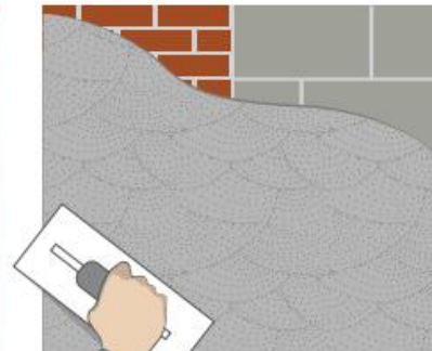
6. Brick or Block Wall Thin veneer stones may be set directly or, a scratch coat of mortar may be applied first to fill in the existing joints and any surface cracks or uneven areas.
