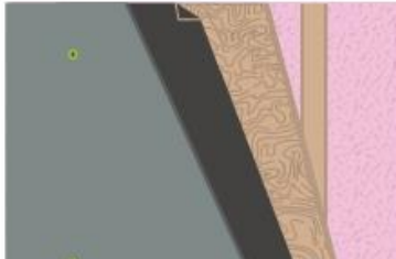
2. Interior Framed Wall - Lath & Scratchcoat Galvanized wire lath is applied directly over sheetrock and felt vapor barrier using waferhead cement board screws anchored into wood or metal studs.
