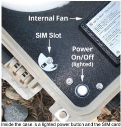
tray. The internal fan helps keep electronics cool if temperatures rise. It is recommended to open the case to help vent excess heat buildup in hot weather.
