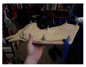
The wire doesn't have to be neat or very tight, it just needs to be secure enough that it isn't exposed when the head is assembled and secure enough that it won't easily be pulled out if someone tugs on the mane.
