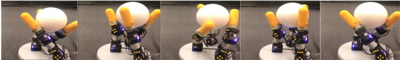
Fig. 3. To demonstrate the feasibility of our designs, we fabricated a hand with 3d-printed parts scaled with regard to the embedded motors. This particular design is meant to rotate a 4 inch diameter ball 180 degrees either way.
