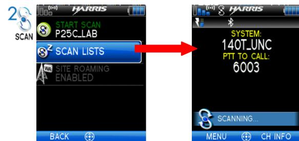
From the **Scan** menu, select **SCAN LISTS** to configure the scan list. Select **START SCAN** to start scan.
