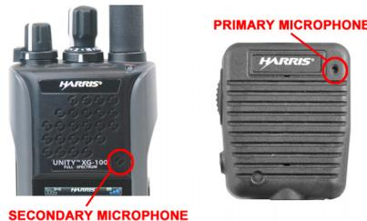
Figure 2: With Speaker Microphone Attached
