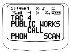
The above screen is typical of what you will see on your radio. The 64 x 96 pixel liquid crystal display (LCD) shows radio status, text, and menu entries.
