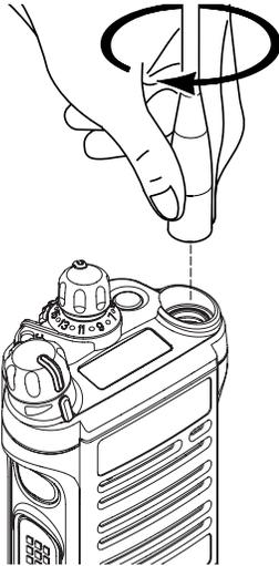
*To remove the antenna, turn the antenna counterclockwise. Make sure you turn off the radio first.*
