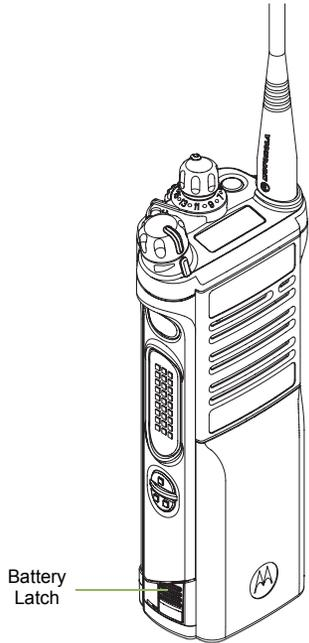
To remove the battery, turn the radio off. Squeeze the release latches on the bottom of the battery until the battery releases from the radio. Remove the battery from the radio.
