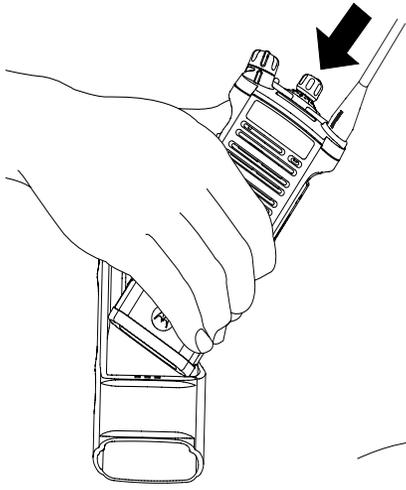
Position the radio within the carry holder with the main speaker facing outward. Slide the radio down into the carry holder until it clicks in place.
