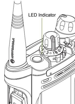
*The LED lights up solid red while the radio is transmitting, and solid yellow when the radio is receiving a transmission (conventional mode only). There is no LED indication when the radio receives a transmission in trunking mode.*
