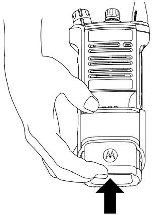
To remove the radio from the carry holder, place the tip of your fingers on the ledge of the carry holder and push at the bottom of the radio until the radio releases from it.
