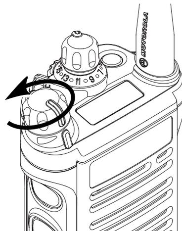
To turn off the radio, rotate the **On/Off/Volume Control Knob** counterclockwise until you hear a click.
