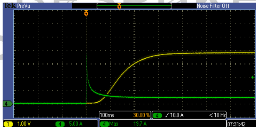
Figure 7. Incandescent Bulb Turn on Current and Optical Output
