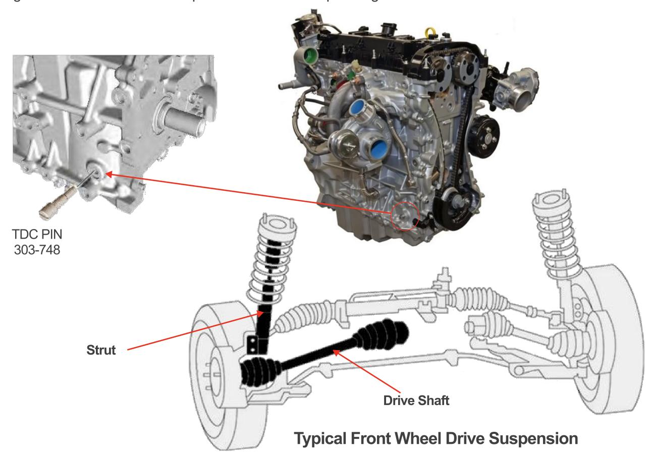
AKABOLT 1AK0010D flexible pin eliminates need to remove any struts or drive shaft to access TDC Pin hole
