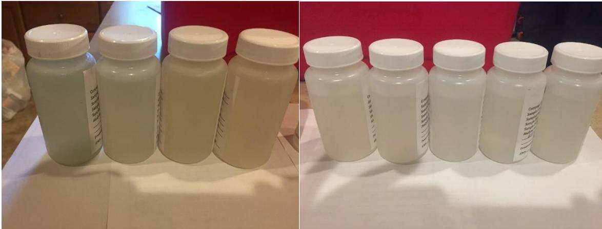
*Above: Water samples sent to Badger Laboratory for testing before and during the WLS system processing. Note discoloration to clear.*
