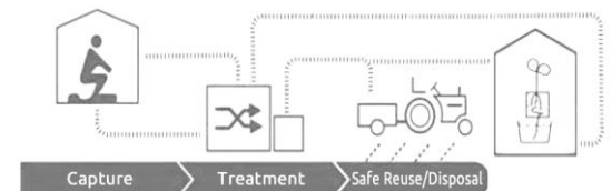
Figure: Water Life Systems reconfigured sanitation service delivery chain that incorporates NSSS/FSTU and container aeroponic farm systems. Shorter chain, resource recovery, reduced carbon footprint.
