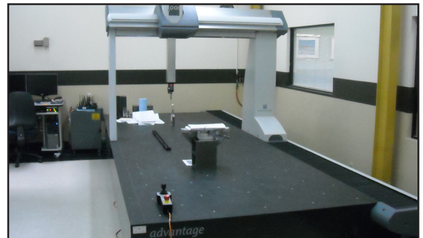
Quality Inspection Dept. CMM Tables
