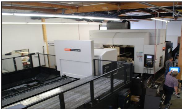
High Speed 5-Axis Mill with Shuttle Changer
