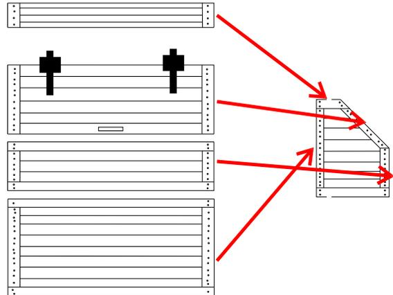
13. Add the stake pockets to the support pieces shown below. Each double dot should match up with a corresponding nipple on a stake pocket. See photos on steps 22 and 24.
