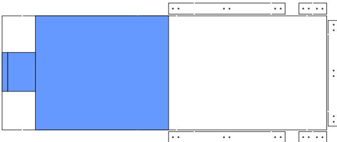
20. Glue the support braces onto the flatbed with the stake pockets vertical on the outside. They are shown sideways in the diagram above for clarity. The opening should allow ladder access. See photos on steps 22 and 24.
