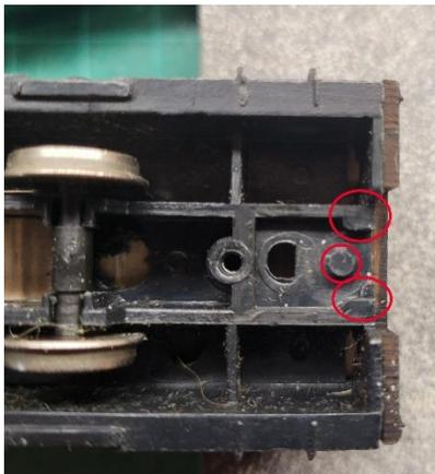
For B – Assemble the coupler box and coupler. Glue it into place using a fast-drying glue. Follow that up with a screw. You may want to pre-drill the hole first. (Shown after installation of the underframe.)
