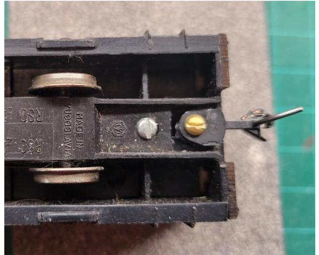
For B and C, cut the underframe with a rotary tool as shown below. Ensure that you cut the correct end.
