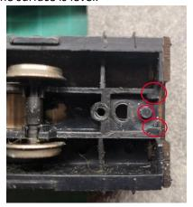
For B – Assemble the coupler box and coupler. Glue it into place using a fast-drying glue. Follow that up with a screw. You may want to pre-drill the hole first. (Shown after installation of the underframe.)
