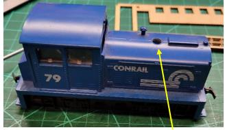
3a. Remove the shell by removing the screw on the top.
