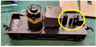
3b. Remove the weight. Use a rotary tool, such as a Dremel to remove the attachment plastic and flatten the bed. The photo below shows where we had added and removed a bed on an early version, which is why there is wood shown.
