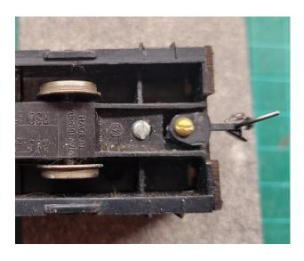
For B and C, cut the underframe with a rotary tool as shown below. Ensure that you cut the correct end.
