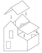
15. Glue the building to the top of the foundation. Overlap should be even on the left, right and rear sides.
