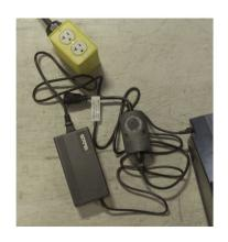
The battery charger is plugged into a timer to avoid overcharging.
