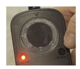
The power light on the timer will come on and the light on the battery charger will turn on, first appearing green and then turning red to let you know it is charging. When the light on the battery charger turns back to green you will know the battery is fully charged.
