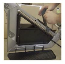
First remove the battery, release the battery stabilizer by pulling out the plunger and lifting up.
