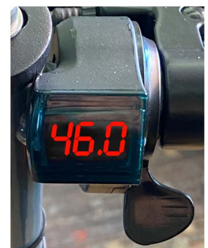
46.0 Volts: Battery is extremely low and essentially dead, though you may get some movement from the cycle.
