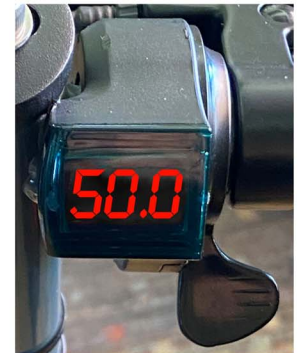
50.0 Volts: Battery is approximately half charged.
