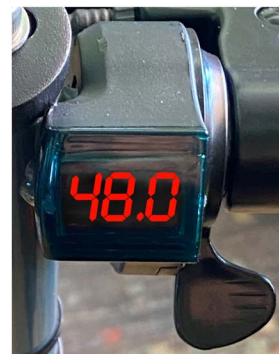
48.0 Volts: Battery is low and needs charging ASAP. For the long-term life of the battery we don't recommend having the voltage drop below 48 volts.
