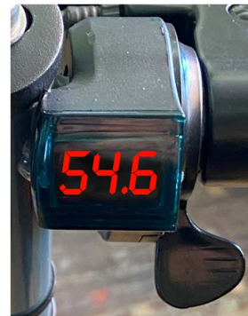
54.6 - 53 Volts: Battery is fully charged.
