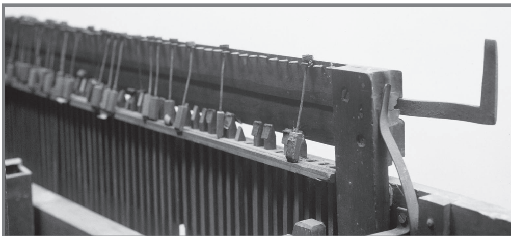
FIG. 13.11. Wood stickers along front edge of case
