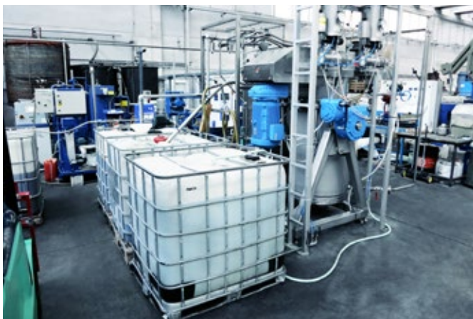
Krauss-Maffei dynamic crossflow filter DCF installation in an oil purification application
