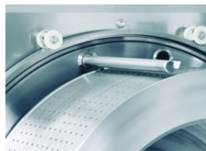
Pneumatic removal of residual heel
